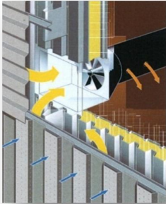
Figure 35 – Concept drawing for transpired solar collector
