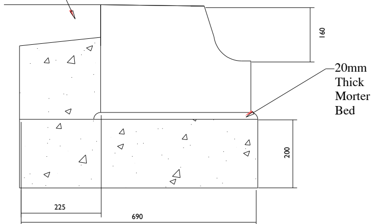
Figure 28.2: Bus Stop Kerb Detail
