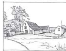
Informal arrangement of steading | courtyard, lean-to's, informal openings, shelter, mature trees, prominent gable with large openings.
