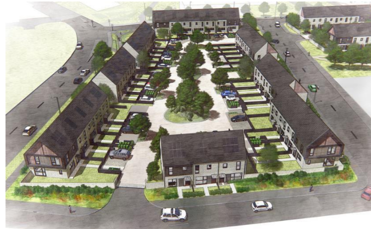
Example of car parking discretely located within a development Commonwealth Games Village, RMJM Architects
