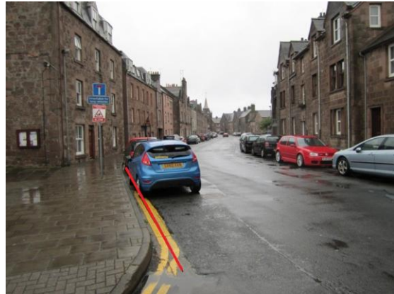
High Street, with linear drain highlighted
