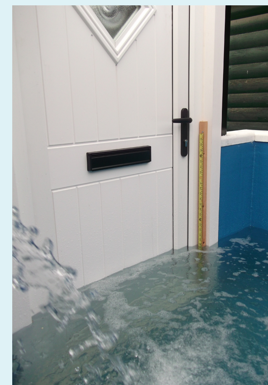
Property Level Protection measures, including [top left, bottom right] door barriers; [top right] temporary barriers, reinforced with sandbags; [below] air brick cover.
