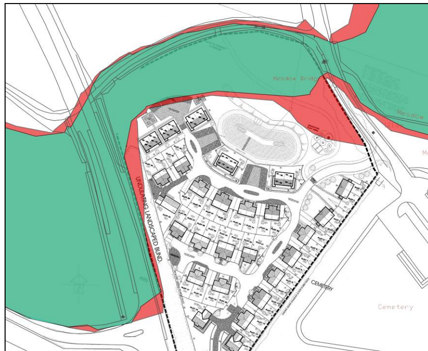
Figure 4-7: Site Layout and original study flood extents
