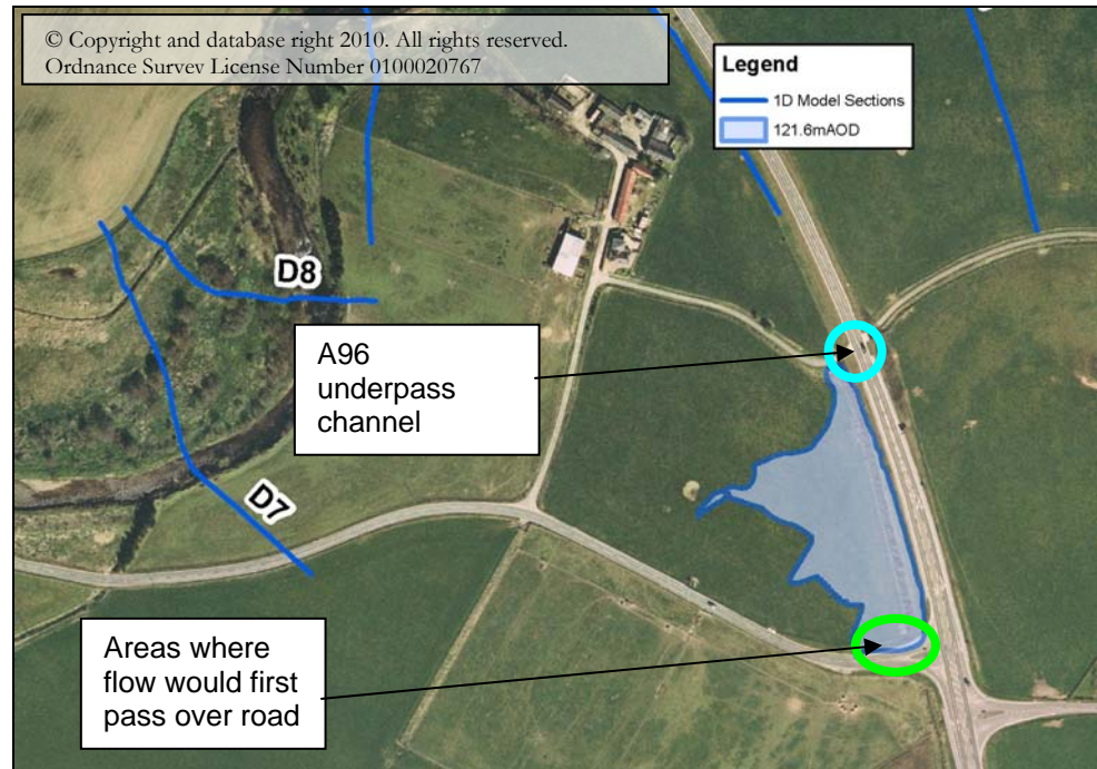
Figure 5-1: Potential Storage Capacity to west of A96
