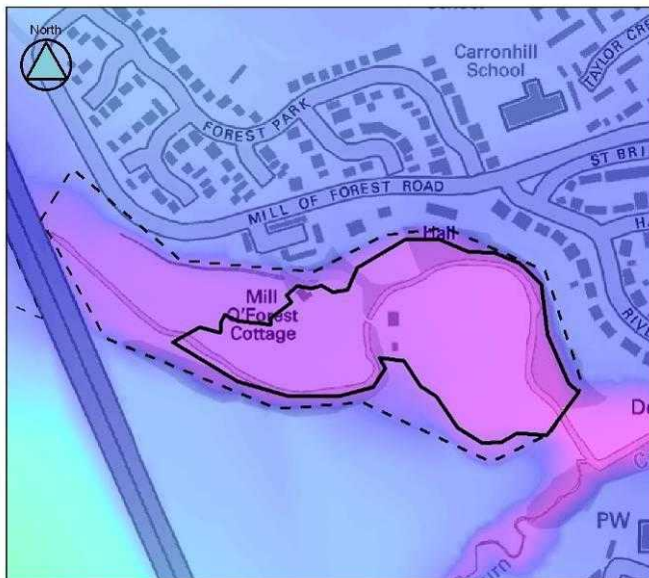
Figure 9-4: Storage area 2 approximate flooded area
