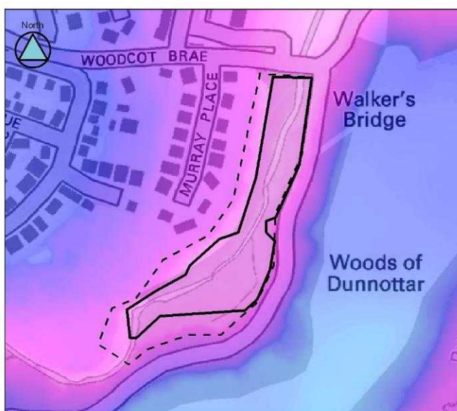
Figure 9-3: Storage area 1 approximate flooded area
