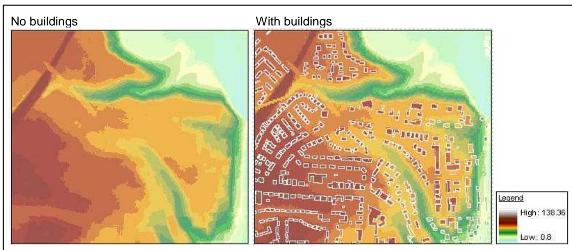
Figure B-4: Adding buildings to the DTM
