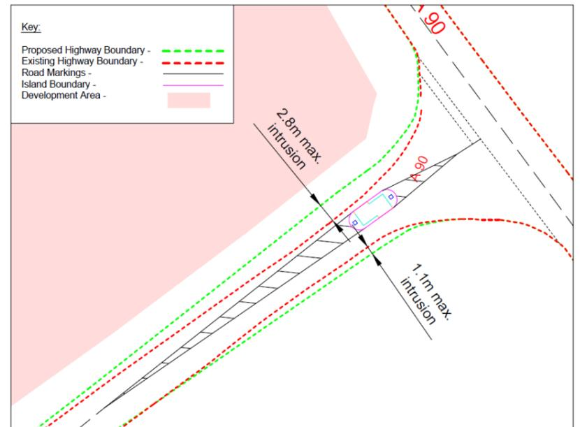
**Figure 12 – Northern At Grade Pedestrian and Cycle Crossing**
