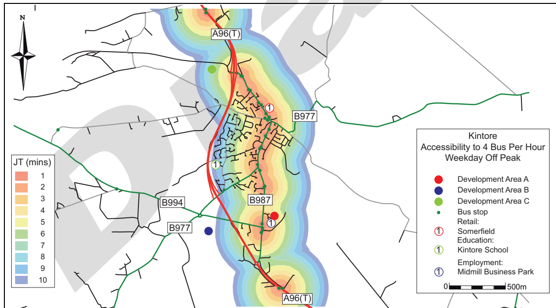
Figure 3.6 : Off-Peak Accessibility to a 15min bus service
