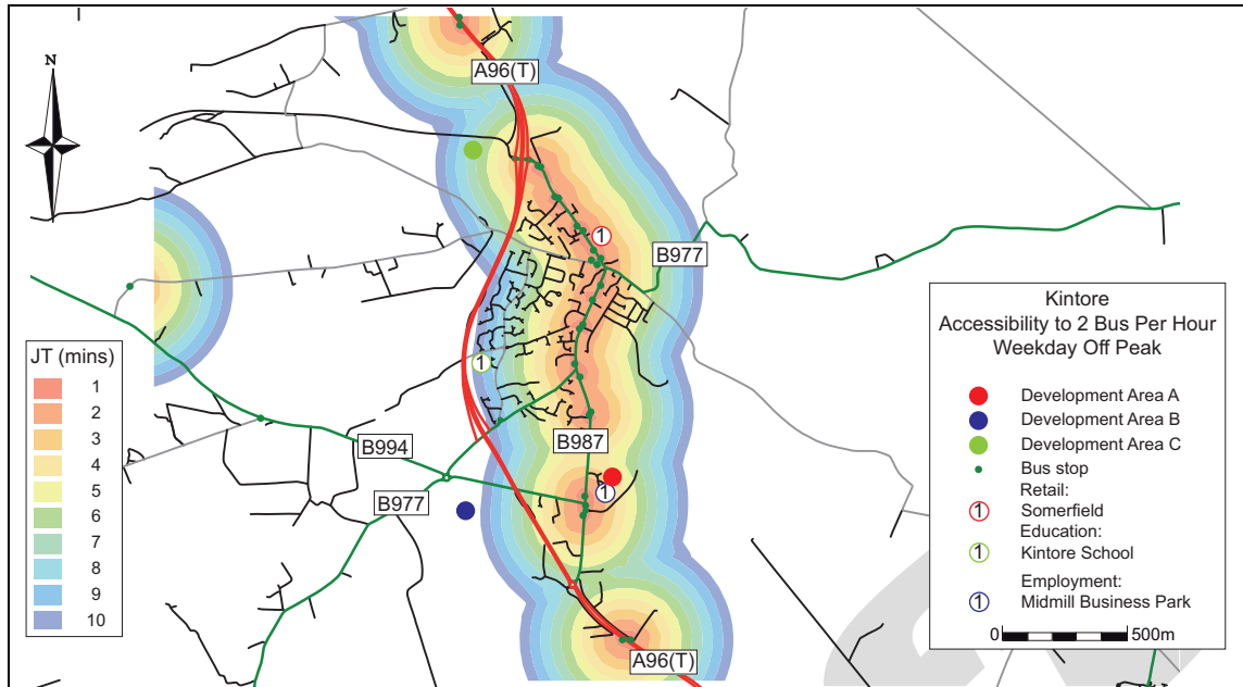
Figure 3.5 : Off-Peak Accessibility to a 30min bus service
