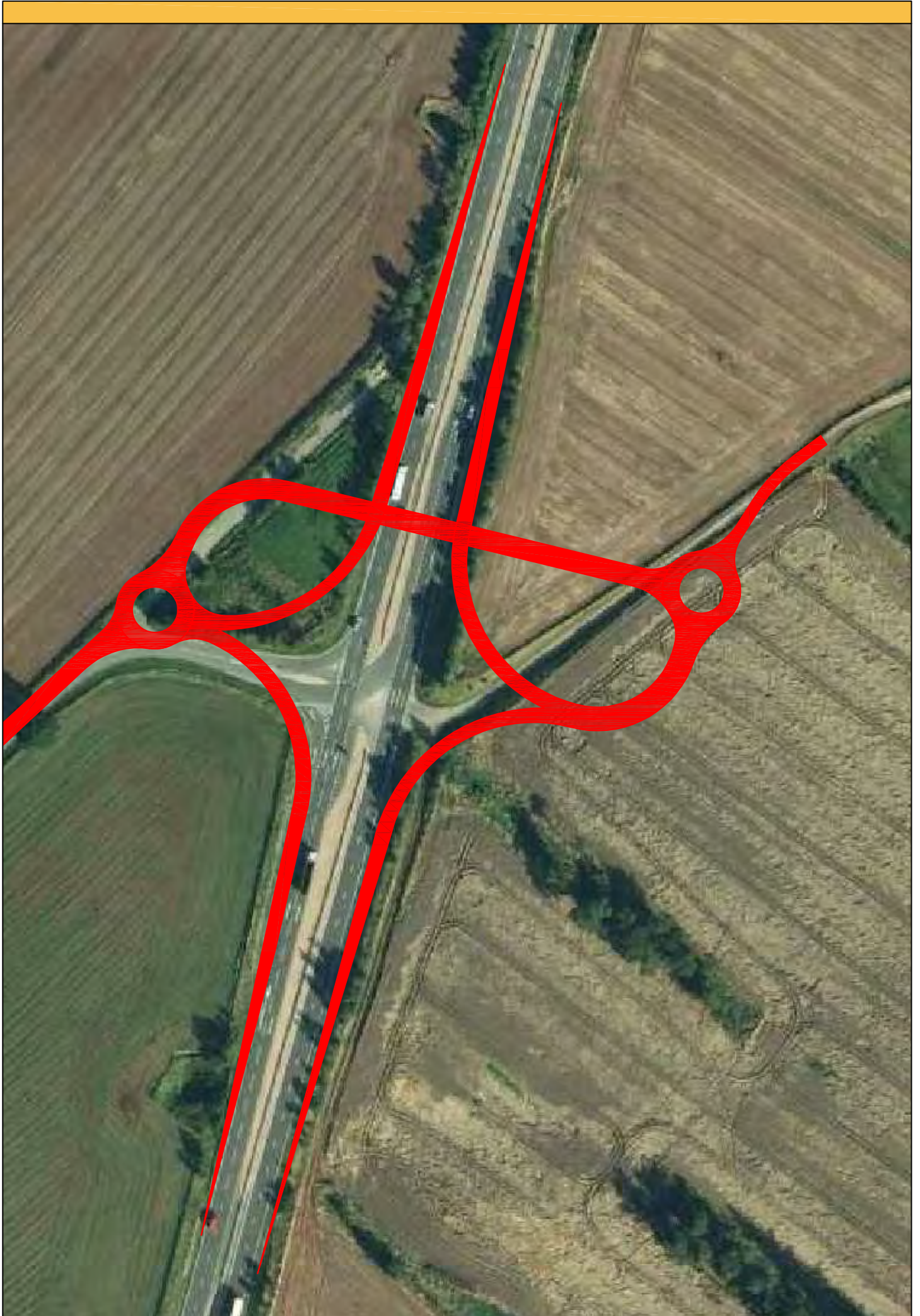
➤ North Junction - Compact Grade Separated Layout
