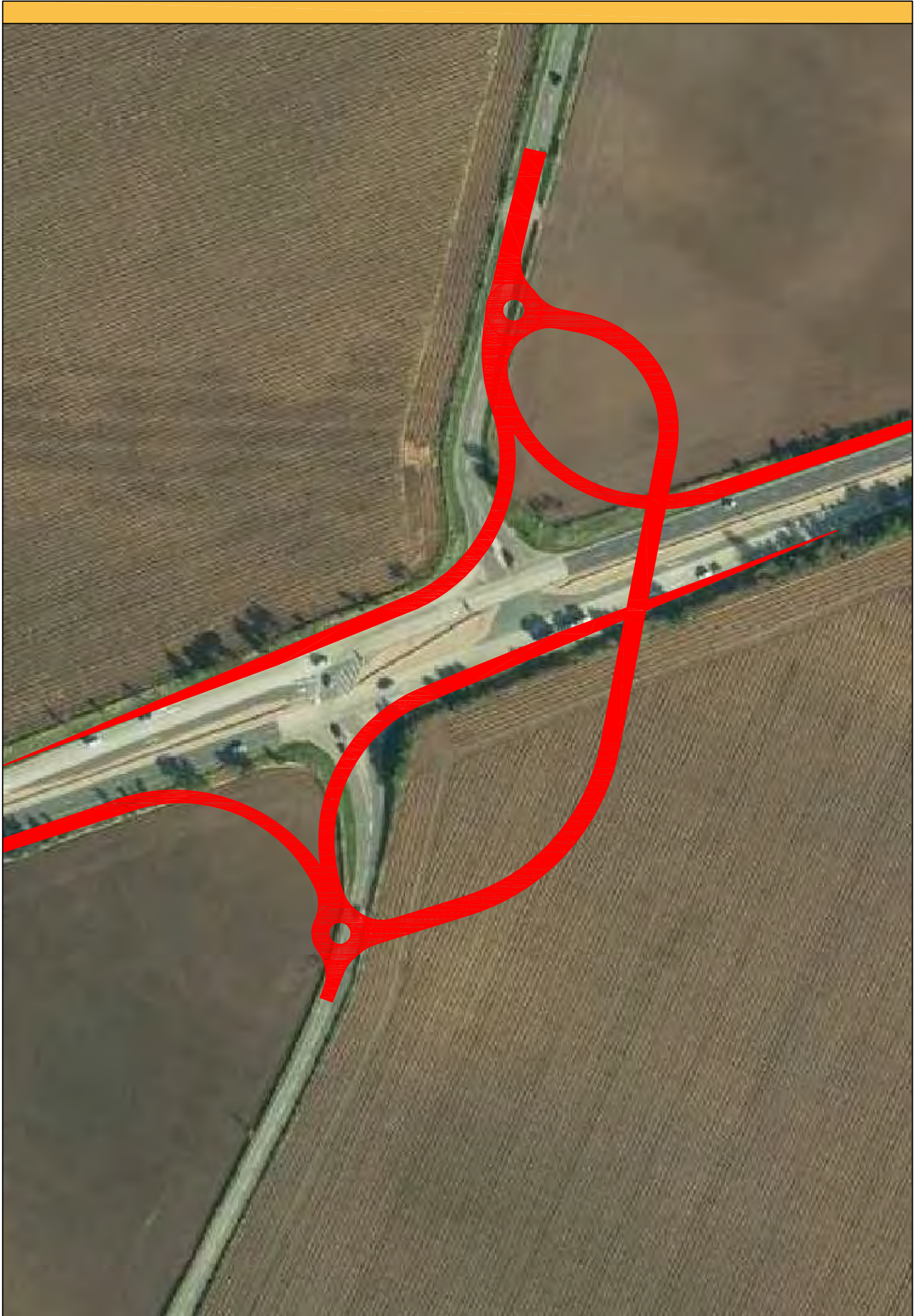
➤ South Junction - Compact Grade Separated Layout
