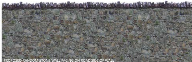
PROPOSED RANDOM STONE WALL FACING ON ROAD SIDE OF WALL
