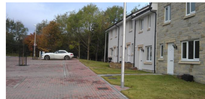
Figure 9: Illustration of shared surfaces
